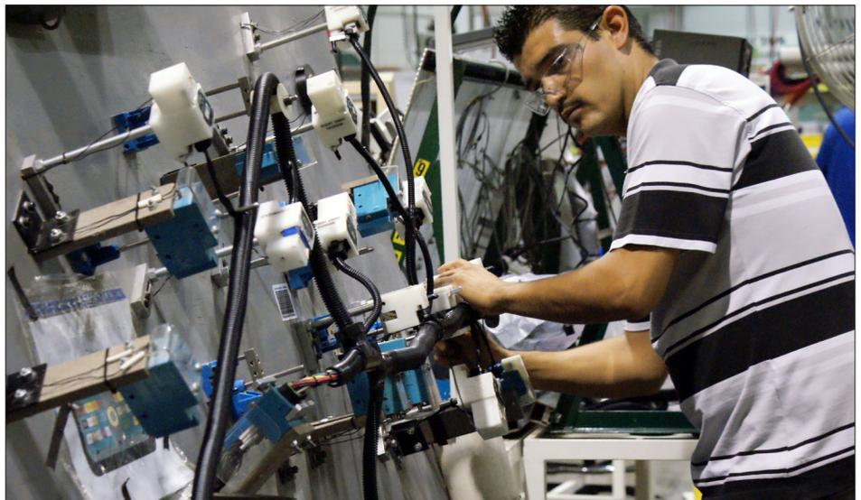
A Group Dekko employee builds an automotive wiring harness. For more than 60 years, Dekko has manufactured components across a wide variety of industries.
